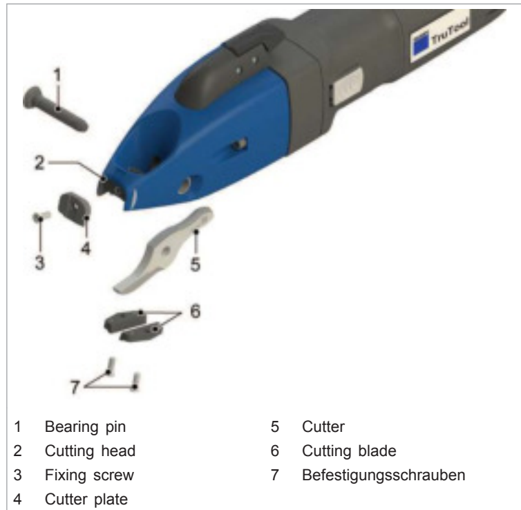
Replacing the tool
